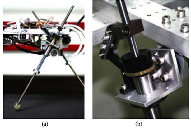
Figure 9. (a) Leg showing compliant spring and angle range, and (b) leg length measurement mechanism design.
