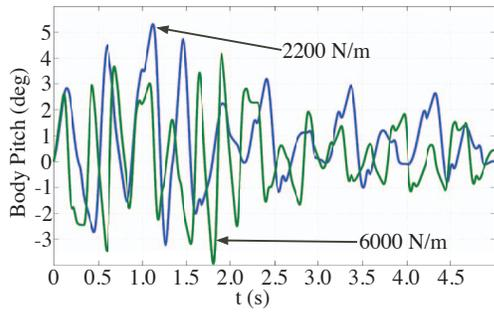
Figure 7. Body pitch for 2200 and 6000 N/m VLeg spring constant.
