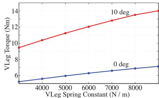
Figure 6. Actuator torque requirements for different VLeg spring constant. Level and sloped terrain.
