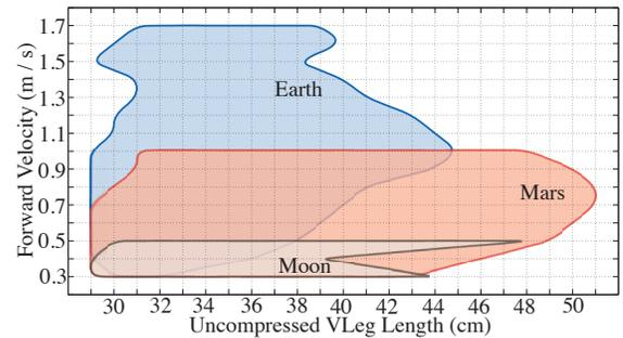
Figure 5. Uncompressed leg length vs. fwd velocity. Level terrain.
