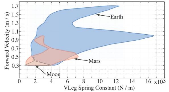
Figure 4. Spring constant vs. fwd velocity. Level terrain.
