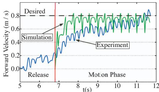
Figure 11. Forward velocity. Simulation and IMU data. Level terrain.
