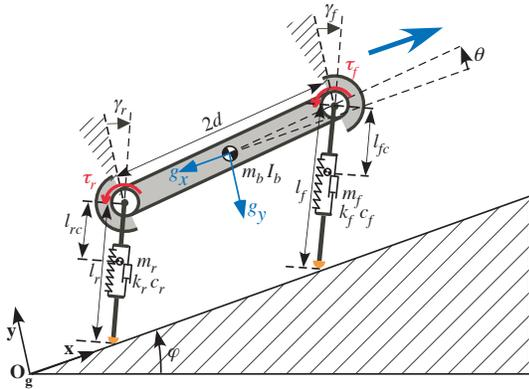
Figure 2. A lumped parameter planar quadruped model.
