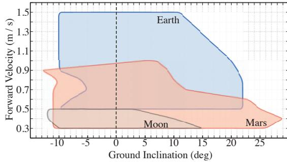
Figure 8. Achievable forward velocity vs. ground inclination for different gravity environments (Earth, Mars, Moon).
